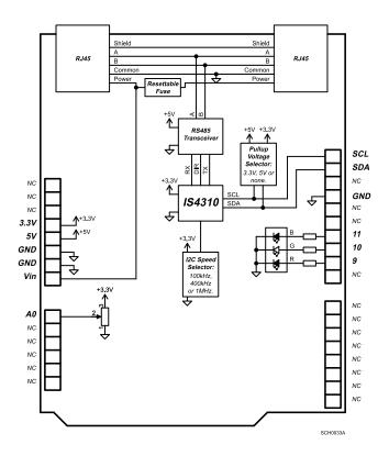
The core of the Kappa4310Ard Modbus Shield is the IS4310 I2C Modbus RTU Server chip, which is connected to an RS485 transceiver. This transceiver interfaces with the daisy-chained RJ45 connectors. Since the connectors are daisy-chained, they are functionally identical—connecting the Modbus master to either one makes no difference.
