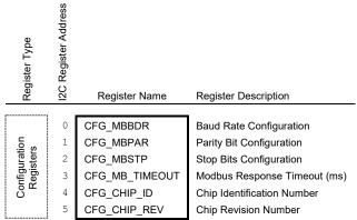
Figure 4: Configuration Registers of the IS4320 Memory Map
