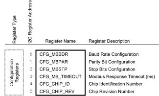
Figure 1: Configuration Registers of the IS4320 Memory Map
