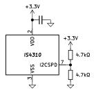
For a 1000 MHz setting, set the I2CSPD pin to 3.3 V.
