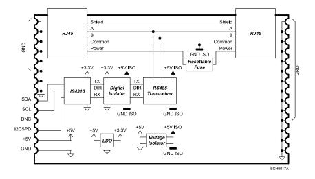
The IS4310-ISO485M6 is a compact (44 × 28 mm) module with castellated holes, designed for PCB mounting to function as an RS485 Modbus RTU Slave. It features two key components: the Modbus RTU Slave Stack (IS4310) and an RS485 transceiver.
