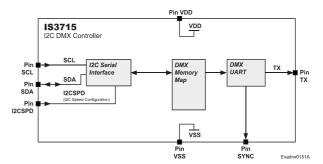
The DMX data is output on the TX pin at TTL voltage levels, while the DMX network requires RS485 voltage levels. Therefore, you must connect an RS485 driver or transceiver, such as the THVD1500, to this pin to convert TTL to RS485. You can find more details about the design in the Hardware Examples section.
