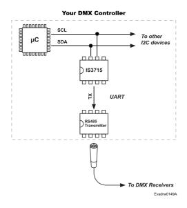
To set the I2C speed, connect the I2CSPD pin to GND for 100 kHz, to 1.65 V for 400 kHz (using a simple resistor voltage divider:  $1.65 = 3.3 \text{ V} \div 2$ ), or to 3.3 V for 1 MHz. The SDA and SCL pins operate at 3.3 V logic levels and are 5 V tolerant.
